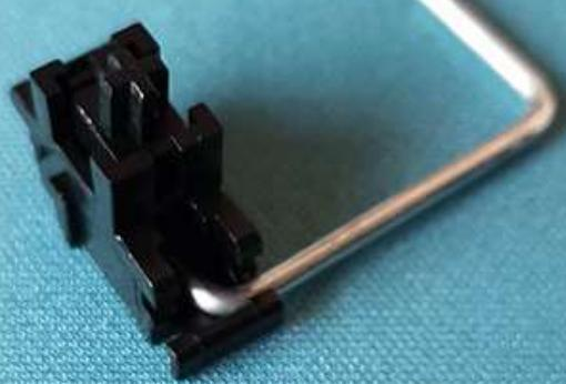
下压钢丝，将钢丝压入槽内，另外一颗卫星轴同理安装钢丝
